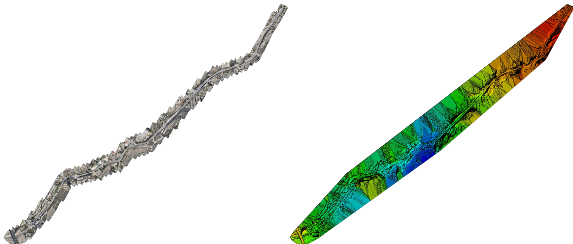
Figure 1: Orthomosaic and the corresponding sparse Digital Surface Model (DSM) before densification.
